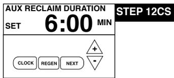
**STEP 12CS** – Only displays if reclamation of brine is enabled in Step 11CS. Use the ▲ or ▼ buttons to select the number of minutes to divert the brine waste water to the brine tank. After the minutes count down to zero the waste water will once again be diverted to the plumbing drain receptacle.
